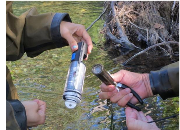
chase four HOBO temperature loggers (above, right). “The temperature loggers are waterproof and record a temperature reading every 15 minutes for up to six years” said Burroughs. “Maintenance is minimal and once a month we simply upload the data to a computer. (picture above, left)”
